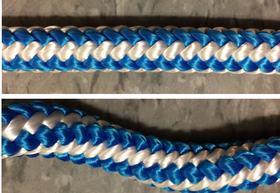
Figure 1: A braided rope where the right-handed and left-handed strands are color-differentiated, showing the interweaving of the two types of strands. When the rope is twisted, strands wrapped in the same direction of the twist (white) become longer and thinner, while strands opposite the direction of the twist (blue) become shorter and thicker.
